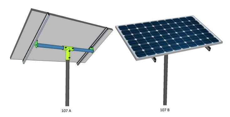
107: Attach aluminum rails to the rail adapter . Install Solar Modules as per Mounting Rail and module manufacturer instructions using top clamps.
