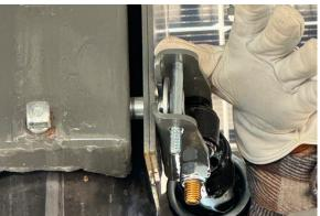
Slide shock bracket under washer and bolt head to the end of the slot in the bracket. Insert keeper bolt into end of shock bracket.
